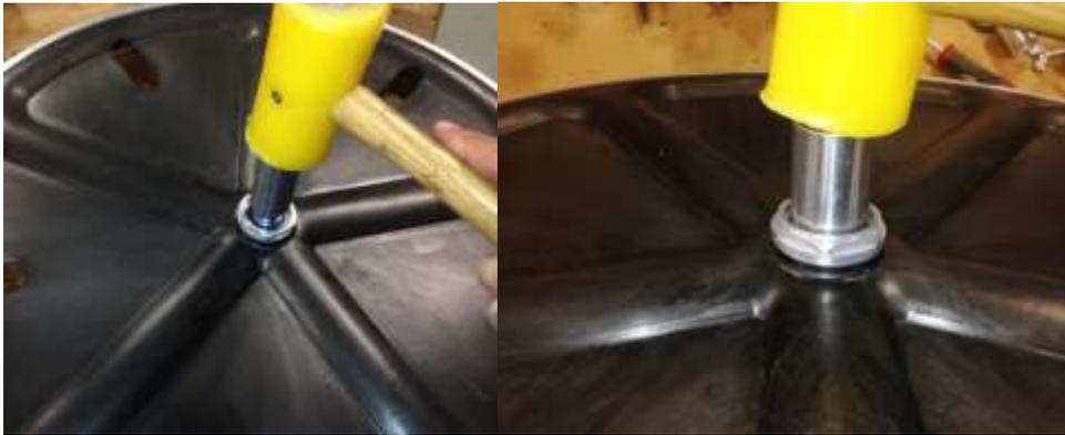
**Step 7:** Place a new bearing onto the end of the hub. Then, while holding the bearing, place the tool kit through the center of the hub and through the center of the bearing on the other side as shown below.
