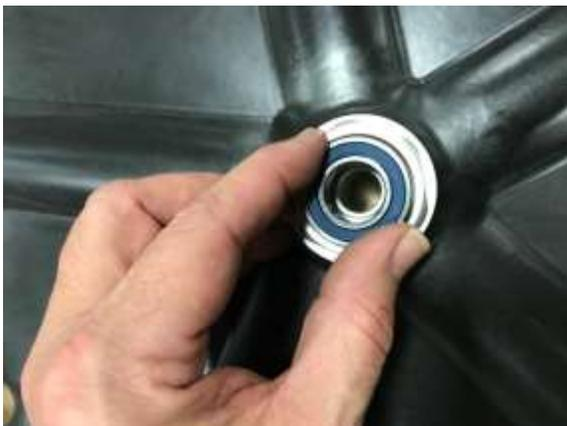
**Step 11: Install stud with large pin through the center of the hub again, being careful not to the axle spacer out of location.**
