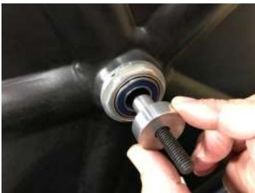
For 4" and 4.6" hubs, place the other nut onto the stud and tighten down with two 11/16" wrenches until you feel the bearing bottom out. Remove washers and stud.
