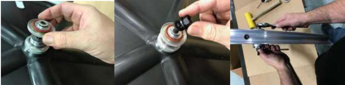
This first tightening operation pulls one bearing into place.
