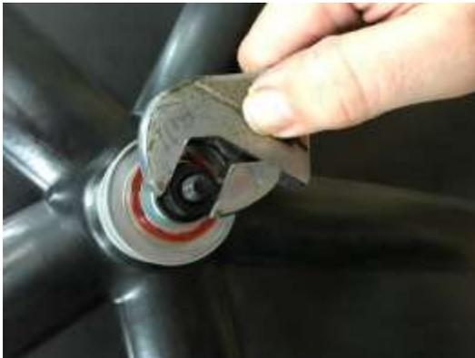
**Step 13: Visually inspect to see that axle spacer is centered in bearings and then install end caps.**
