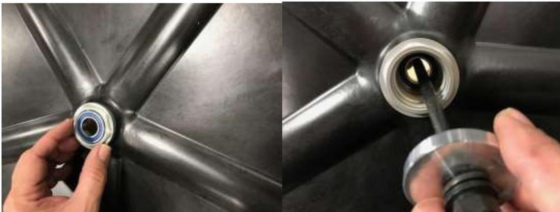
**Step 8:** Place the smaller diameter washer/pin from the kit over the stud as shown.
