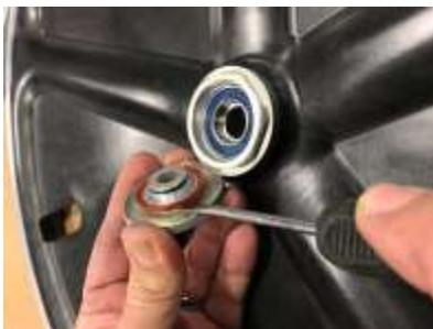
**Step 4: Clean off the end caps and install the new seals (and new O rings in groove, if needed) as shown below. Make sure to press the new seals all the way down until they bottom out. \*NOTE: Some older generations of end caps may be slightly too large to fit the new seals. If this is the case, simple do not use the seals. The bearings themselves are sealed. Be careful not to rip the seals when installing.**
